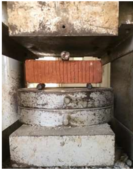
Figure 6. Flexural strength test for specimens
