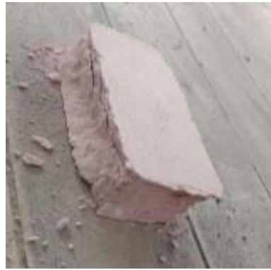
a) Failure of Autoclaved aerated concrete (AAC) blocks b) Failure of solid sand-lime bricks
