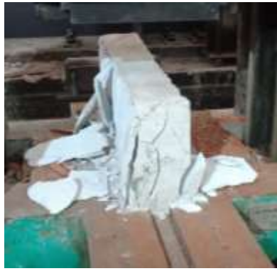
a) Failure of Autoclaved aerated concrete (AAC) blocks b) Failure of solid sand-lime bricks
