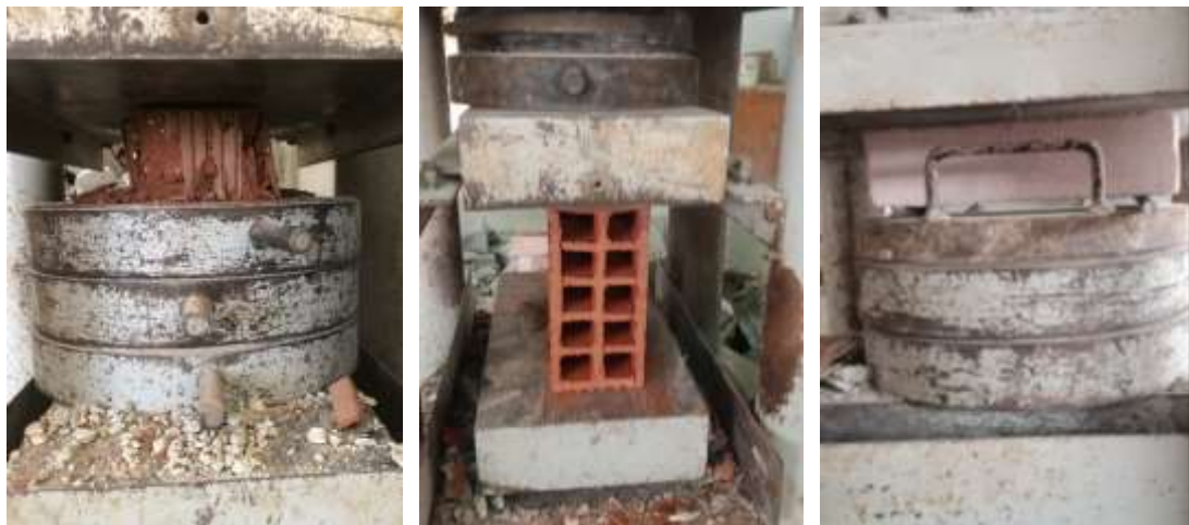
a) first-class perforated clay brick unit subjected to compression test
