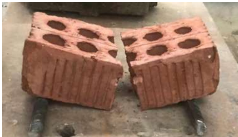
a) Failure of first-class perforated clay brick unit
