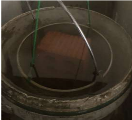
Figure 9. Second-class perforated clay brick immersed in water for 24 hours
