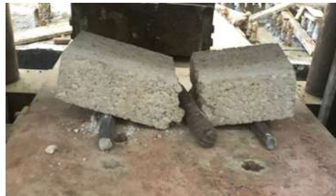
b) Failure of first-class solid cement brick unit
