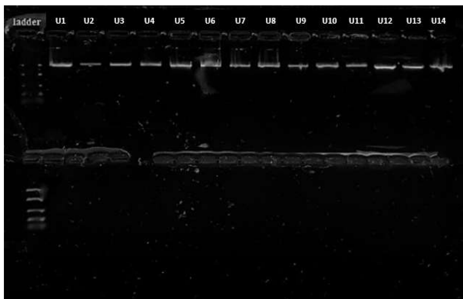
Figure 2: Band visualization under UV after gel electrophoresis (samples U1-U14)
