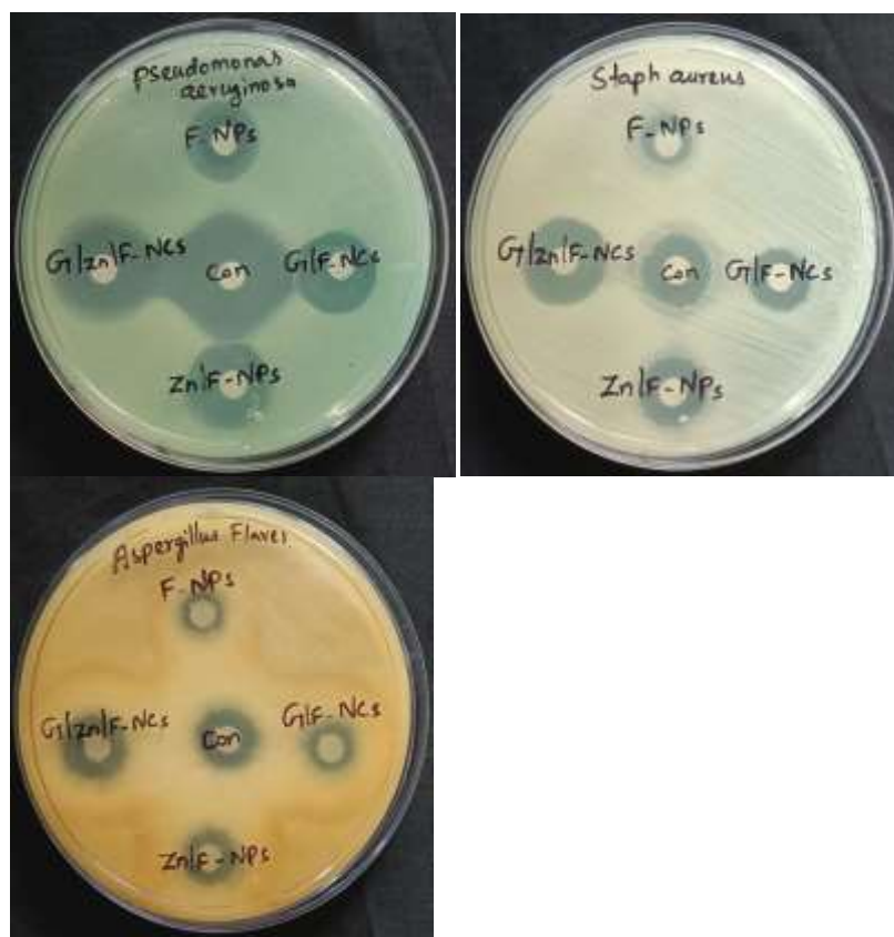
Figure 9 illustrates the ZOI of F-NPs, G/F-NCs, Zn/F-NPs and G/Zn/F-NCs for Pseudomonas aeruginosa , Staph aureus , and Aspergillus flavus
