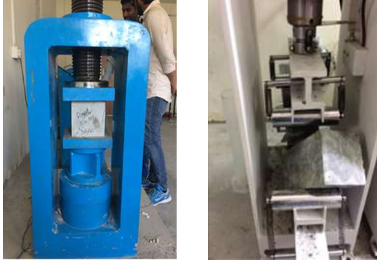
Fig-01: Compressive strength & Flexural strength test of concrete clicks.
