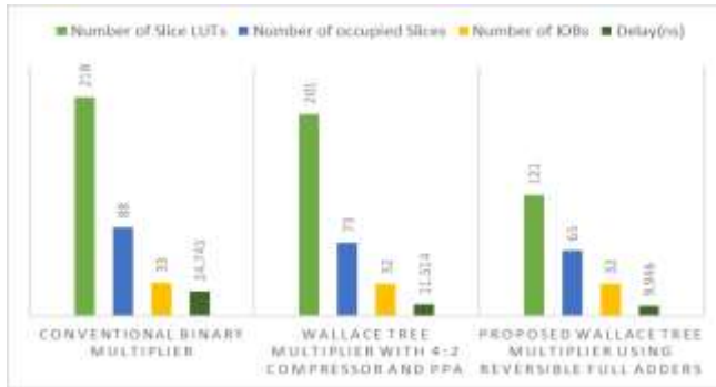
Figure 5: Xilinx results analysis graph of proposed, existing wallace tree multiplier with conventional binary multiplier
