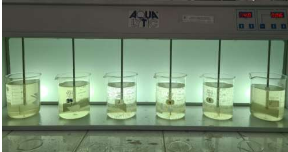
Fig. 7 Figure VI.5 Jar Test Comparison of PAC and CBBN-dw (Left-Right: 1-6)
