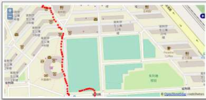
Fig 5. Trip converted to sequence of network edges using map matching
