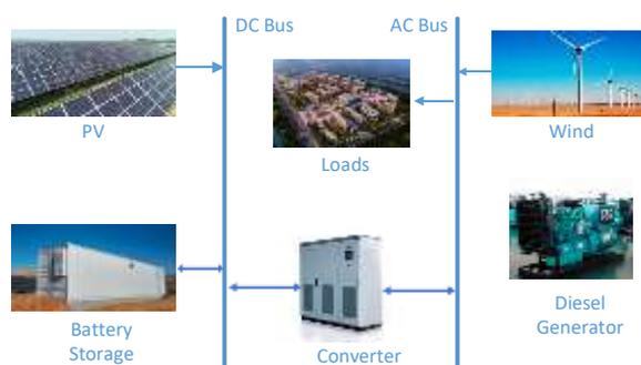
**Figure 1** Configuration of wind-solar-diesel-battery system
