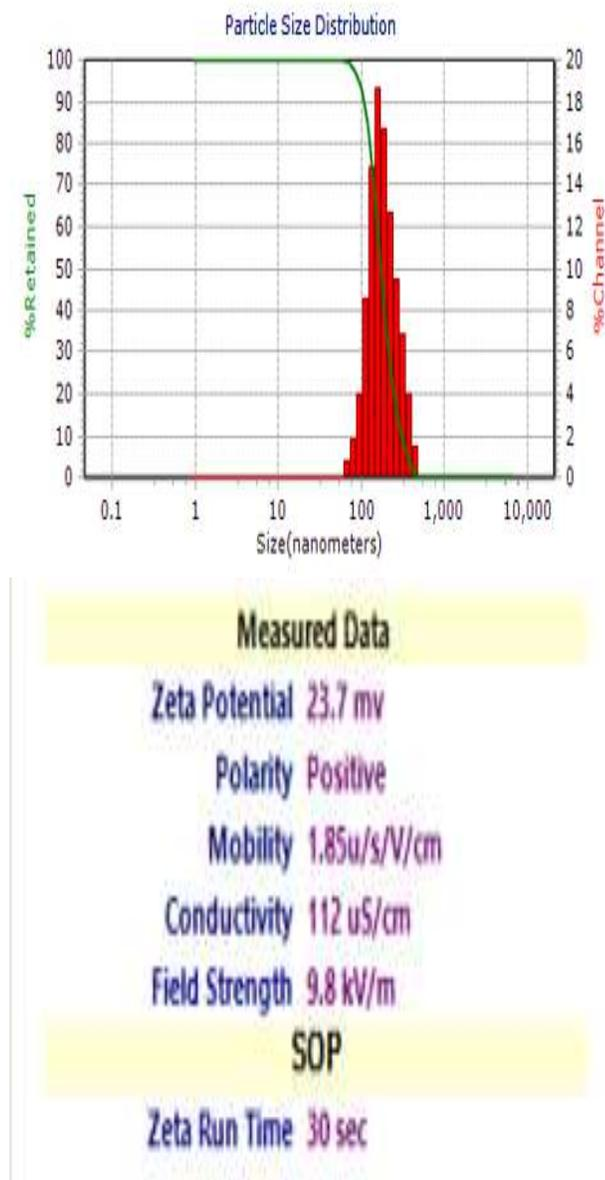
**Figure 3:** shows the synthesis of three different AgNPs in various concentrations of *G. asiatica*, according to a 0.1 molar solution of silver nitrate. The sizes ranged from 80 nm to 500 nm. All samples exhibited a low polydispersity index (PDI) of 0.46, 0.54, and 0.35, with a Zeta potential value of 23.7mv.
