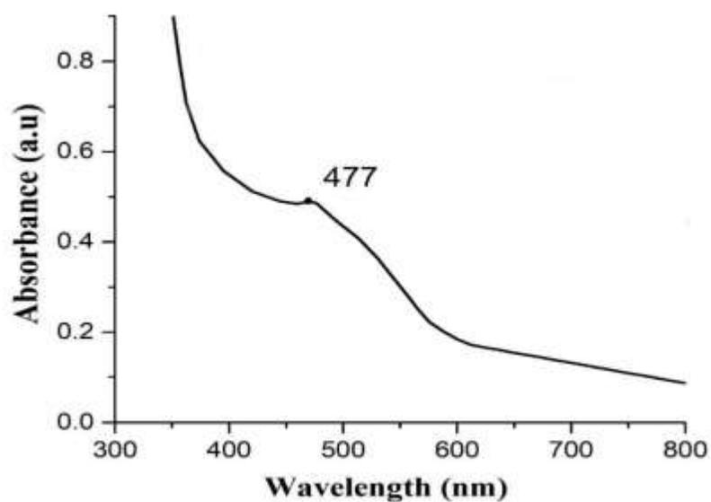
**Figure 2:** displays spectroscopy, utilizing a peak in the range of 400-500nm to validate the production of AgNPs. The wavelength of the instruments used fell between 200-800nm, and *Grewia Asiatica*-mediated AgNPs exhibited a wavelength range of 435-477nm.
