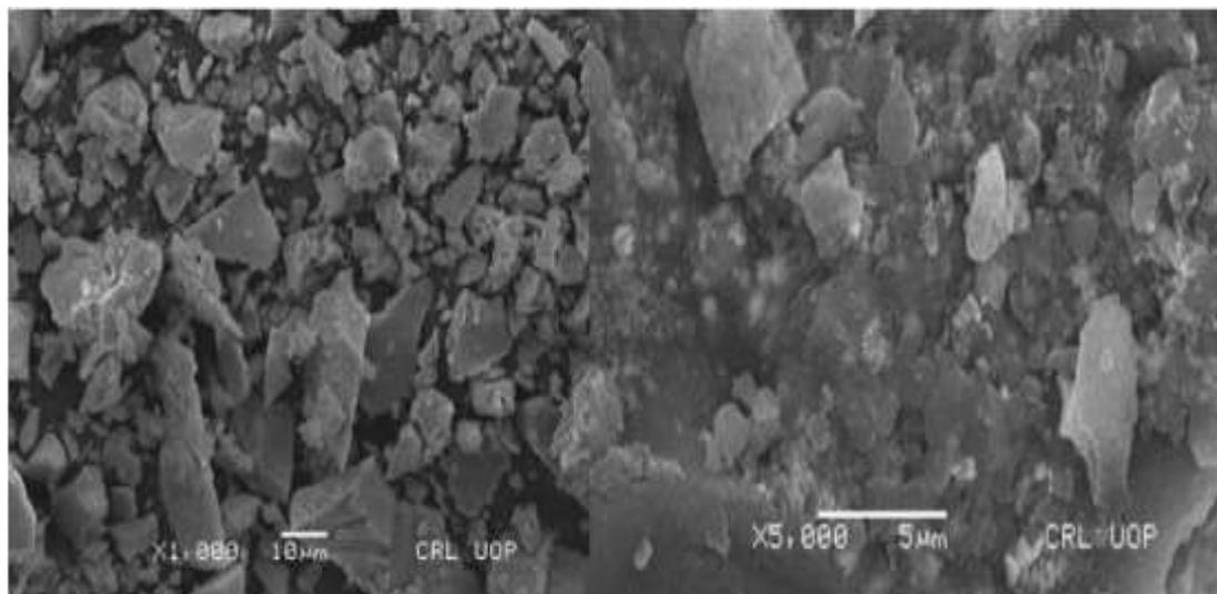
**Figure 6:** SEM images of green synthesized Ag-NPs obtained by *Grewia Asiatica* extract at room temperature (It was revealed that some silver nanoparticles were clumpy (cluster), and other were spherical. Some particles seem to be large, while others appear to be tiny in size. The morphology of the nanoparticles which vary in size from 72.7 to 239.1nm.
