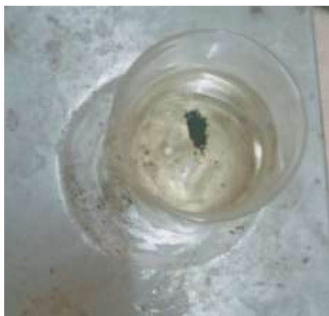
Figure 2. Graphene oxide nanoparticle mixed with polyolester oil
