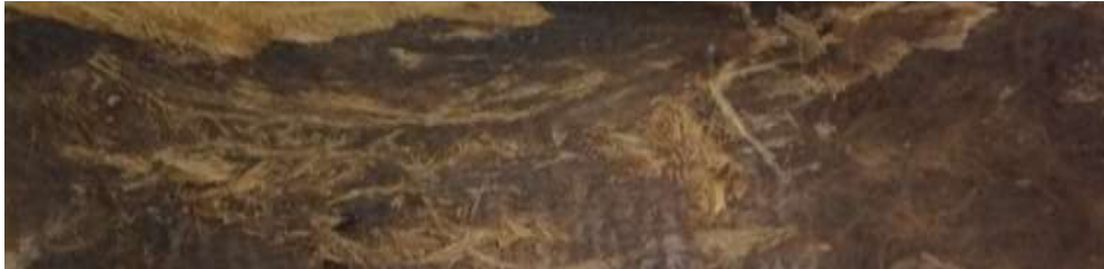
Fig.3 Sample (78 Epoxy resin- 20 jute fiber- 2 Boric acid)
