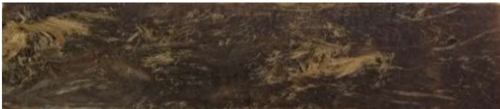
Fig.4 Sample (77 Epoxy resin- 20 jute fiber- 3 Boric acid)
