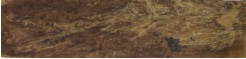
Fig.2 Sample (79 Epoxy resin-20 jute fiber-1 Boric acid)
