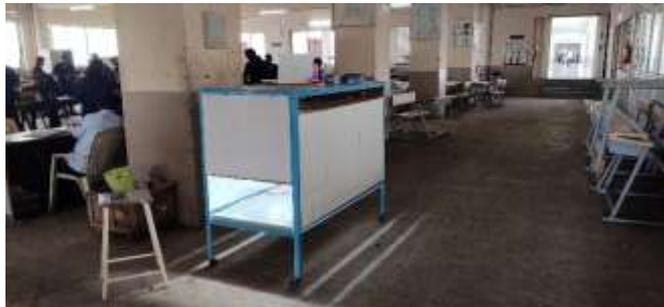
Above fig shows Performance Simulation with in house solar panel setup, which is consisted of four main parts: solar PV module, Light bulbs module, reflectors and electrical module. The PV panel heated by halogen bulbs radiation will be resulted in an increase of the temperature of PV cells. Meanwhile, the heat transferred by the PV to PCM can be absorbed. Then, the decrease in temperature will results in improved performance [12].
