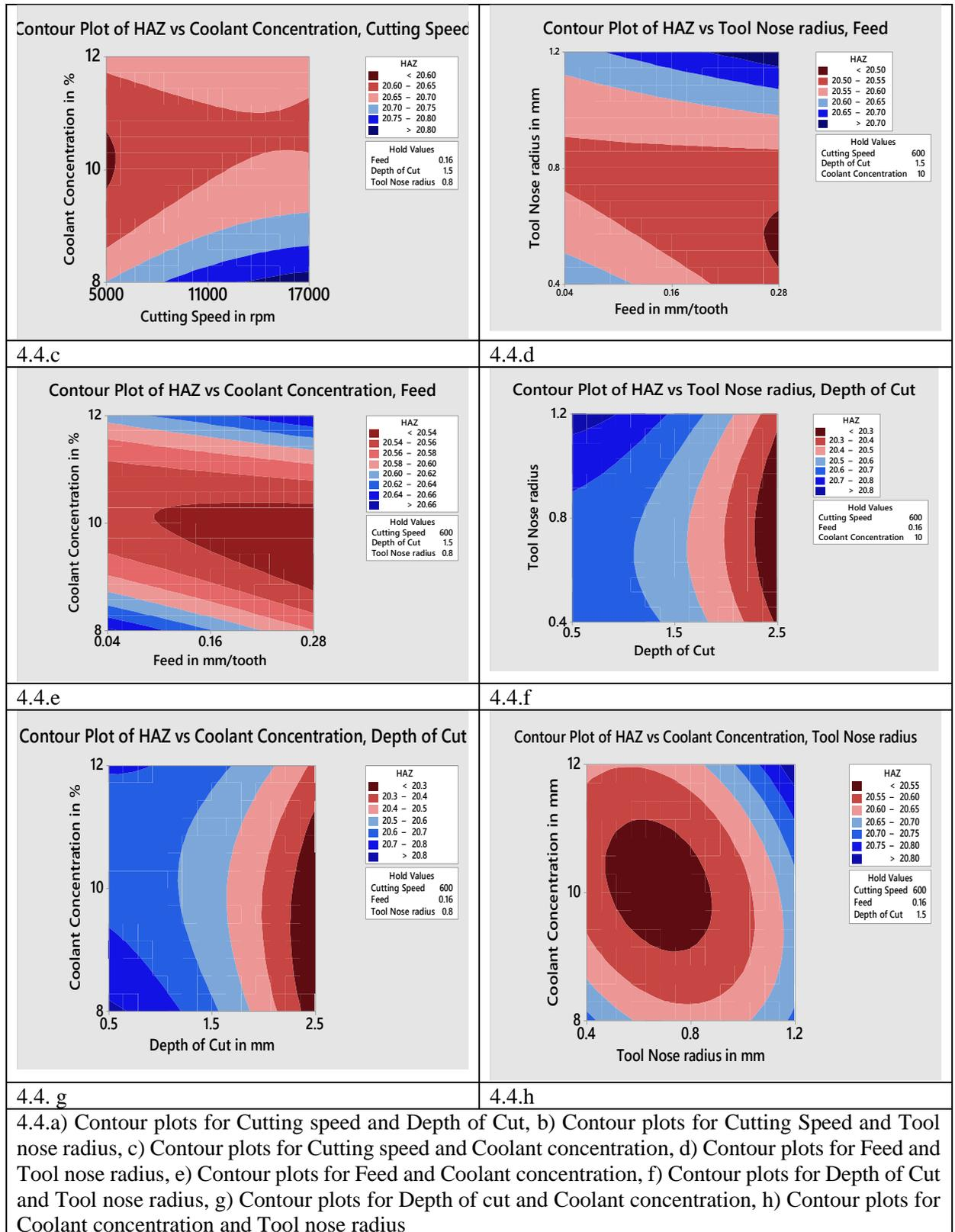
Fig 4.4.a – 4.4.h represents the contour plots for interaction between cutting speed, feed, depth
