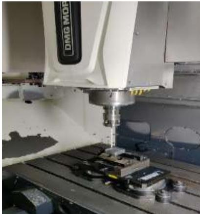
**Fig. 7:** Experimental set-up of the milling of a sample specimen
