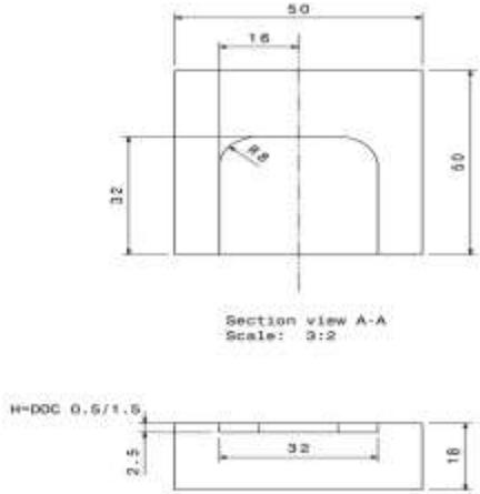
**Fig 3:** Sample specimen drawing of size 50 x 50 x 20 mm
