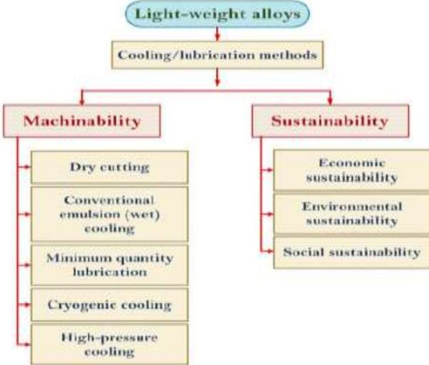
Fig 2: Coolant strategies and methods for light weight alloys [28].
