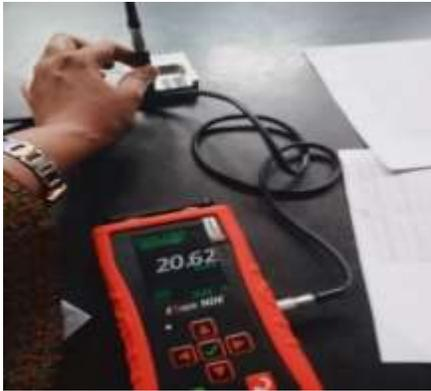
HAZ measurement using Eddy current meter on Sample specimen
