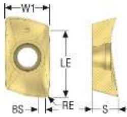
**Fig.4:** Seco Insert Carbide Uncoated from XOEX10T3
