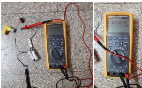
Figure 12: Discharging of batteries at a time gap of 1 hour
