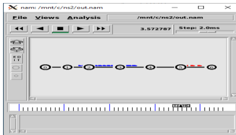
Figure 3: Network with 7 nodes in simple linear architecture
