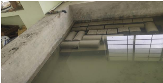
Figure 4: GC cubes and cylinders in the curing tank
