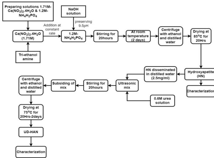
Figure 1: Synthesis of HAN and UD-HAN using sol-gel method
