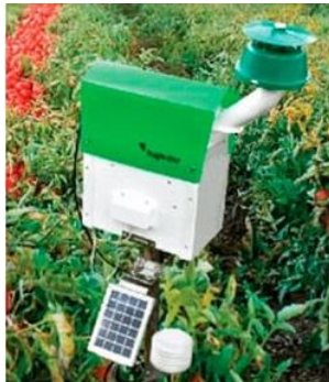
Image 3. Sensors to Trap Fruit Flies (Cardim Ferreira Lima et al., 2020)
