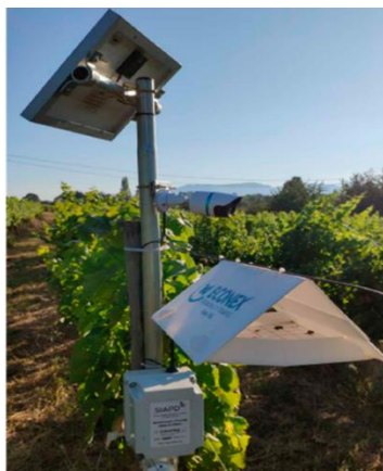
Image 4. Devices installed to collect images of grape moths (Teixeira et al., 2023)
