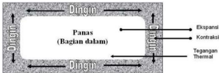
Figure 1. The phenomenon of "Poor Thermal Conductivity"
