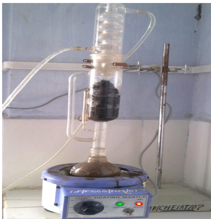
Figure 2.1: Soxhlet apparatus showing extraction.
