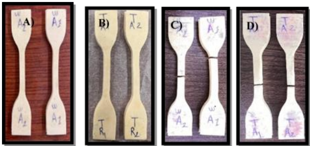
Fig. 2: Test Samples of Tensile testing (A, B-before test, C, D -after test)
