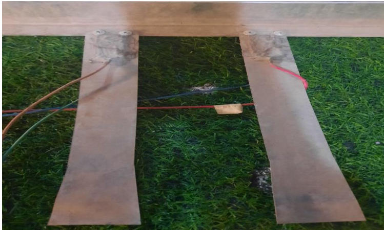
Figure (5): the smart cantilever beam.
