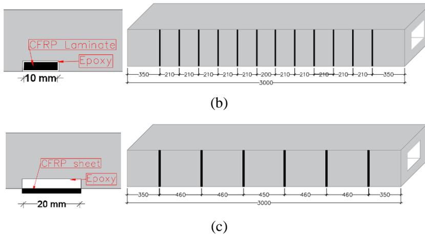
Figures 3. (a) NSM-CFRP on two sides, groove width=20 mm (NL-20), (b) NSM-CFRP on two sides, groove width=10 mm (NL-10). (c) EBROG on two sides with one layer width=20 mm (EBS-S).
