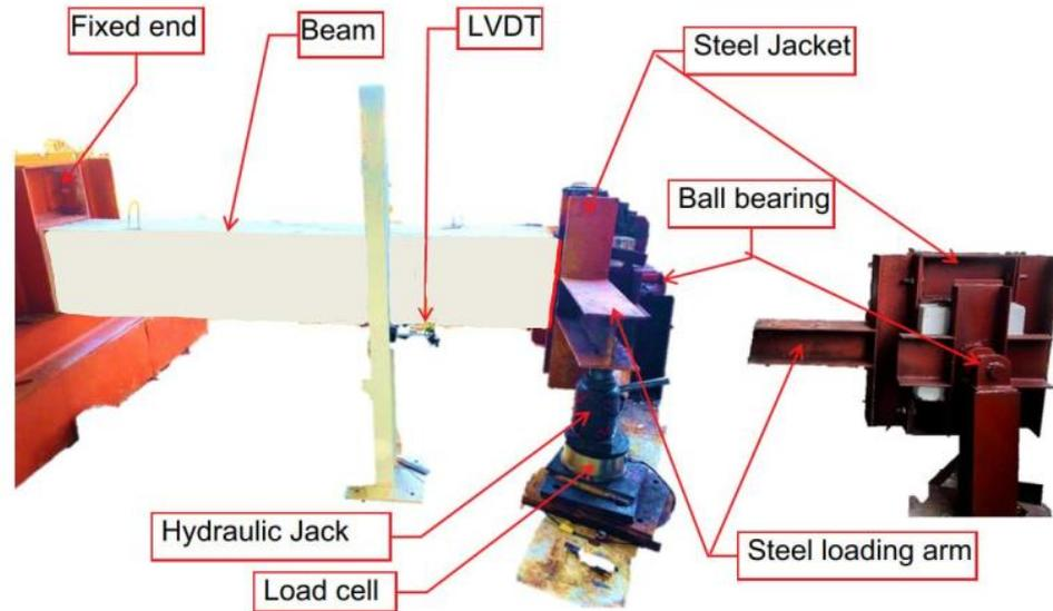
Figure 5: Torsional test systems
