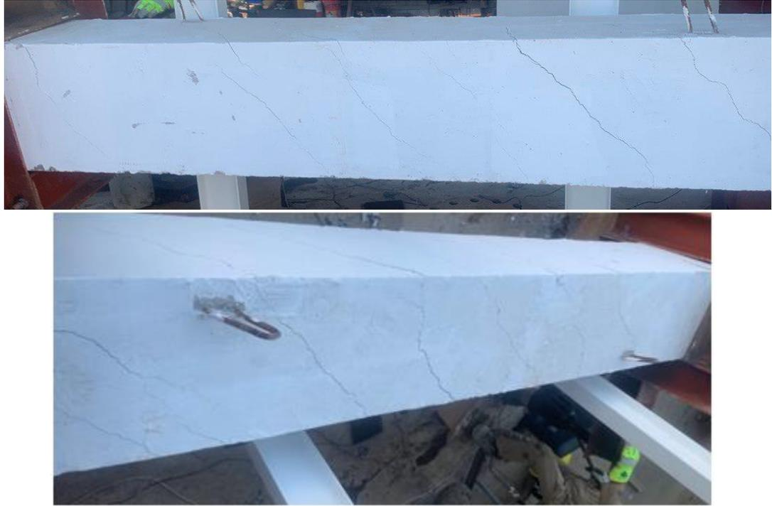
Figure 9: Strengthened beam NL-20 failure and crack configuration.
