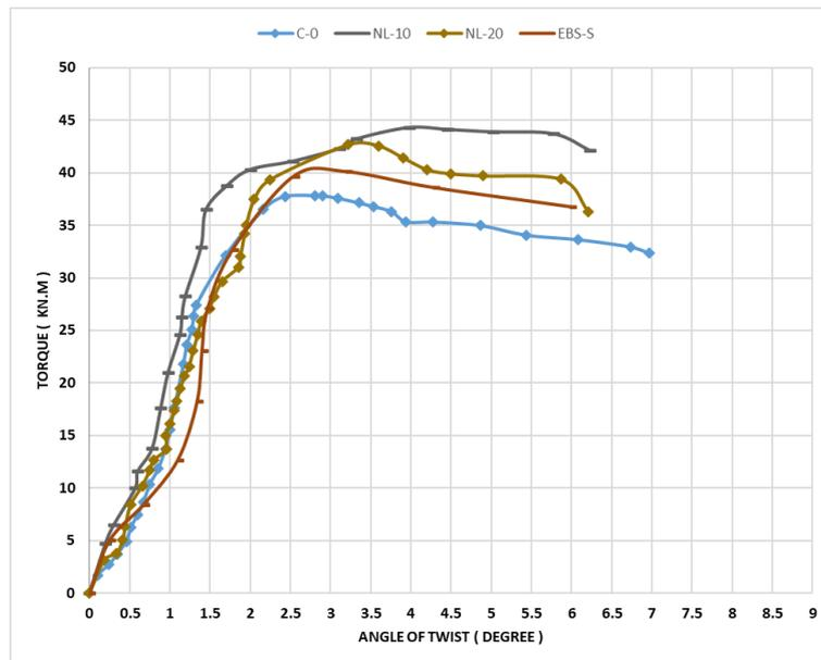
Figure 6. Torque-twist curve of the beams that were tested.
