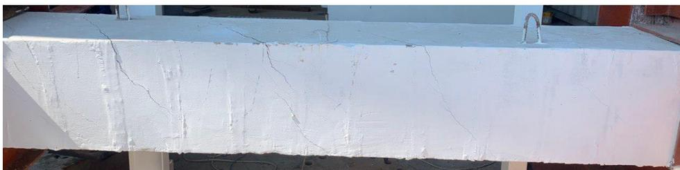
Figure 8. Strengthened beam NS-10 failure and crack configuration
