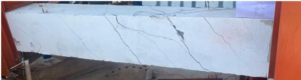
Figure 7: Control beam (C-0) failure and crack configuration
