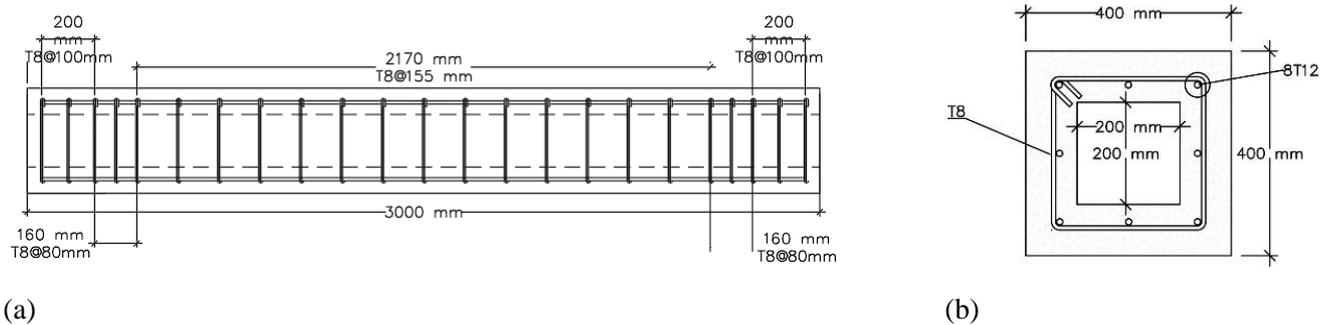
Figure 2. beams details: (a) longitudinal -section of beams; (b) the cross-section of beams
