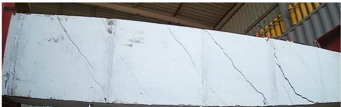
Figure 10. Strengthened beam EBS-S failure and crack configuration.
