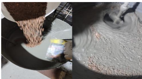
Plate (3-16): LECA is added to the mixture
