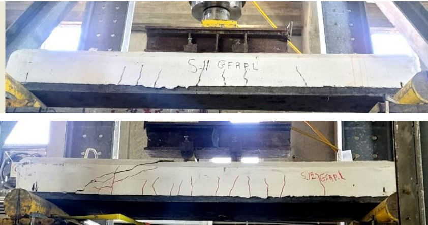
Figure (7to 12) Crack patterns of Slabs (S4to S12)
