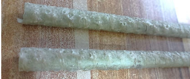
Fig. 1: The Geometry of GFRP Bars Used in This Work
