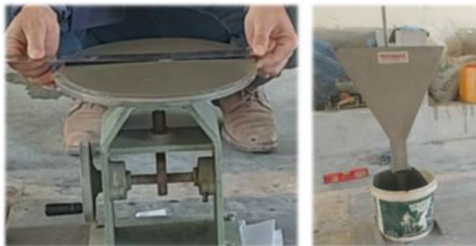
Figure (4): Tests for SIFCON mortars using miniature slump flows and V-funnels
