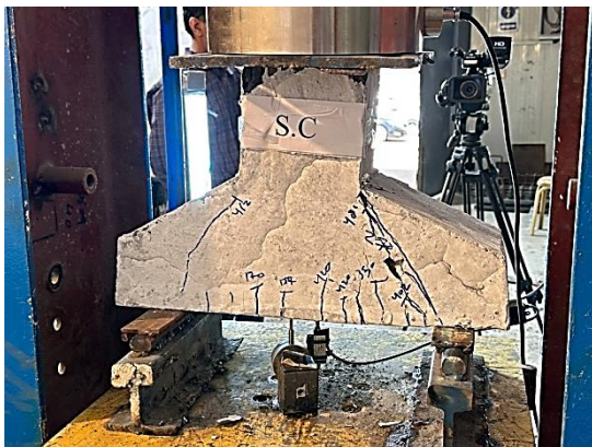
Figure (14) Full SIFCON Specimen (failure mode)
