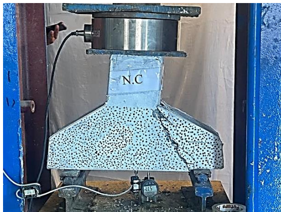
Figure (12) Normal Concrete Specimen (failure mode)
