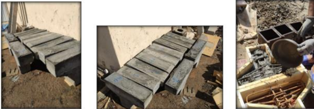
Figure (10): Casting and Curing the specimens
