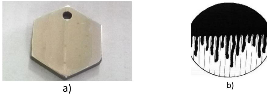
Figure 5 - Sample with HCN coating (a); diffusion along the microcrack grid (b)
