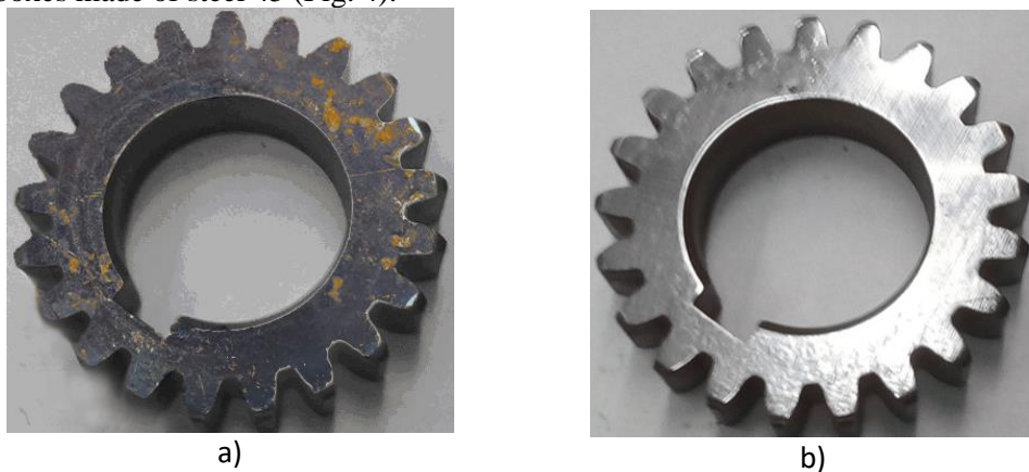
Figure 4 - Gear subjected to corrosion (a); gear restored with the help of HGDN (b).
