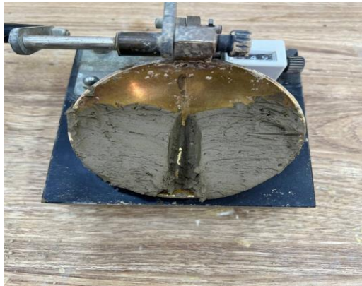
Figure (2): liquid limit test.
