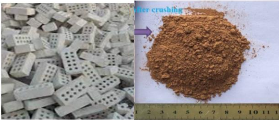
Figure. (6): brick used for this study after crushing
