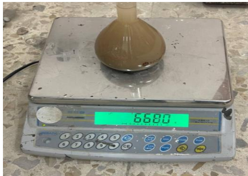
Figure (3): Specific Gravity Test.
