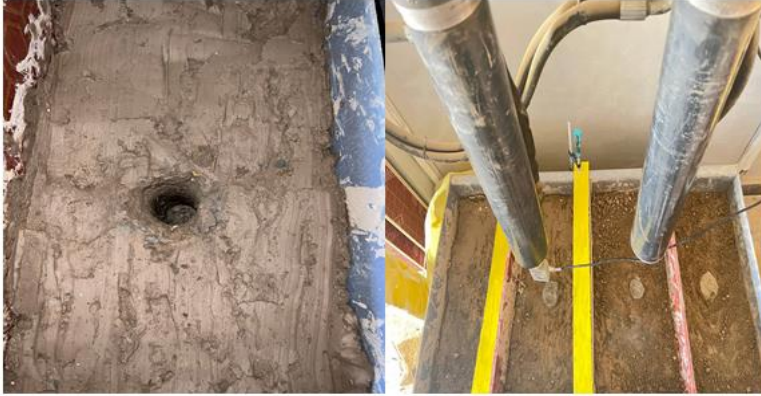
Figure. (9): Preparation sand column.
