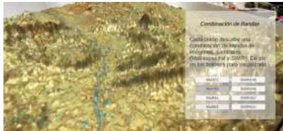
Figure 8. View of the processed DEM and then converted into a 3D object in AR with the 753 combination, fake standard color. Band Combination: Each button describes a combination of satellite imagery bands (multispectral and SWIR). Click on the buttons to view it. Source: The Authors
