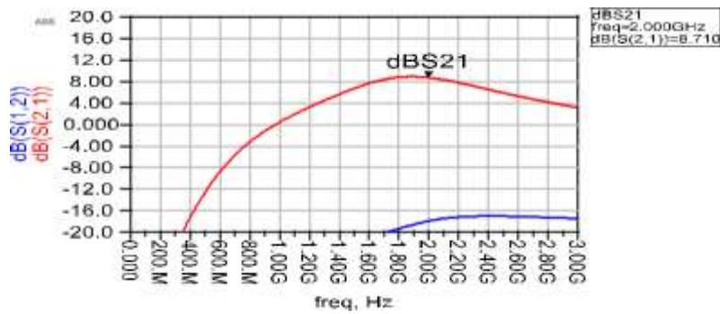
Figure 4: Frequency response of amplifier gain
