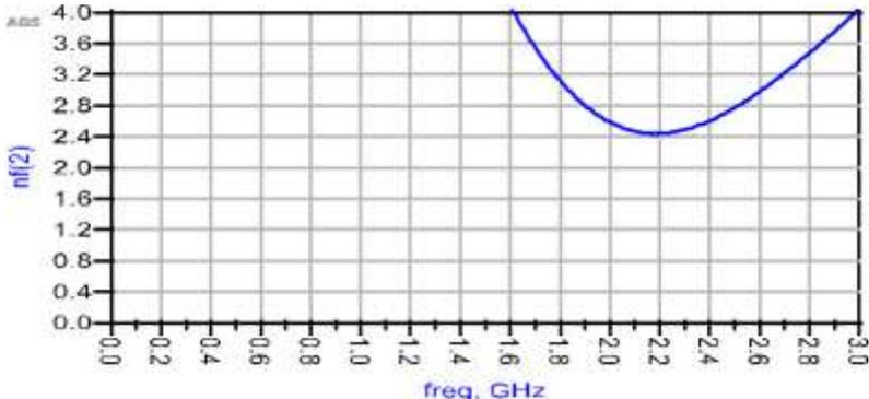
Figure 9: Noise efficiency factor response of Amplifier with input and output matching networks
