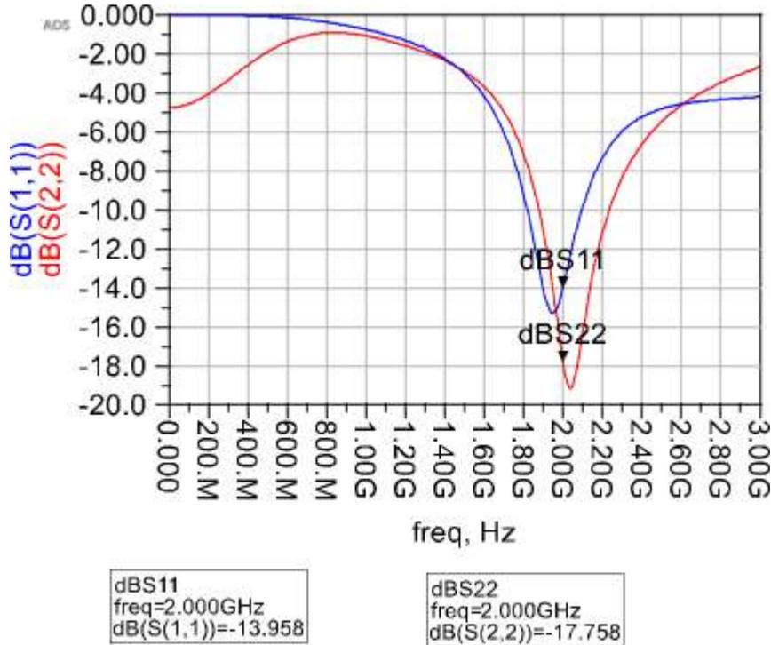
Fig 8: Amplifier with stabilization, input, and output matching components added
